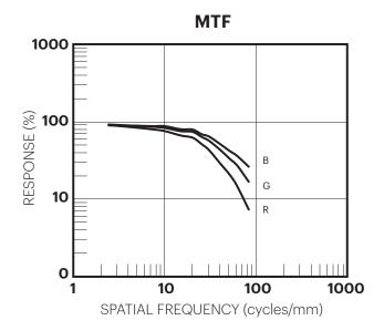
MTF curve - This graph shows a measure of the visual sharpness of the film. The x-axis, "Spatial Frequency", refers to the number of sine waves per millimeter that can be resolved. The y-axis, "Response", corresponds to film sharpness. The longer and flatter the line, the more the film can resolve, and therefore, the sharper the film.
